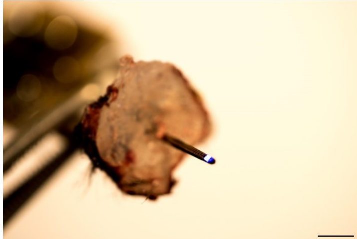
Supplementary Fig. 12: Image of a wireless photometry system operating after implanted in BLA region for 2 months. Scale bar, 2 mm.
