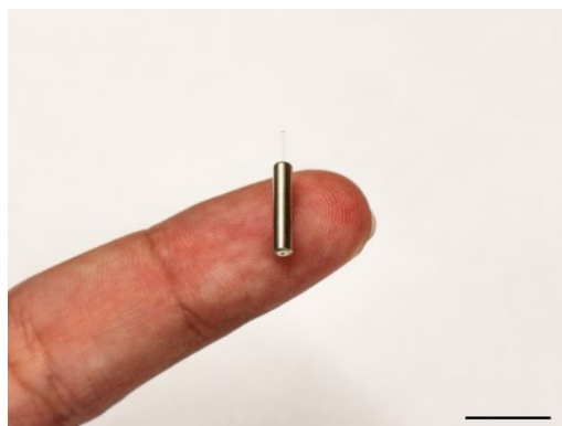
Supplementary Fig. 5: Image of an optical cannula on a fingertip. Scale bar, 12 mm.
